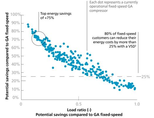
22 kW, 7 bar example based on real customer data
