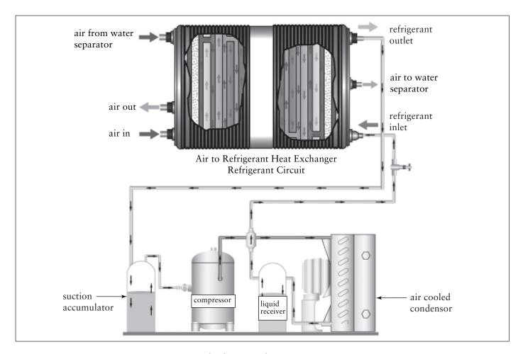
Typical Schematic Flow Diagram
