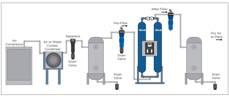
FIGURE 3-1: Typical Installation Setup
