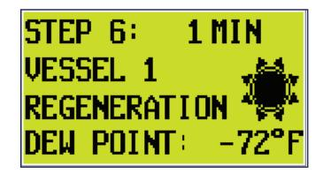
FIGURE 5-19: Step Six Heating
