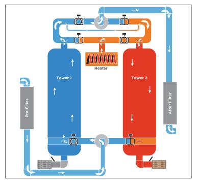
FIGURE 2-1: TYPICAL SCHEMATIC FLOW DIAGRAM AEHD Series 150 - 3,000 scfm rated model
