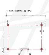
REMOTE CONTROL PANEL WITHOUT SPACER MOUNTING HOLES
