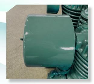
Quiet Intake Filter Oversized air filter reduces noise level of the air compressor
