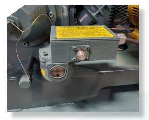
Low Oil Control Protects the compressor pump from damage due to lack of lubrication
