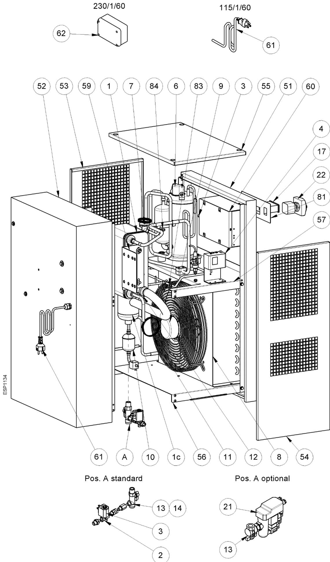
13.2.6 Exploded diagram DRYPOINT RS 180-350 HP50 NA Water-Cooled
