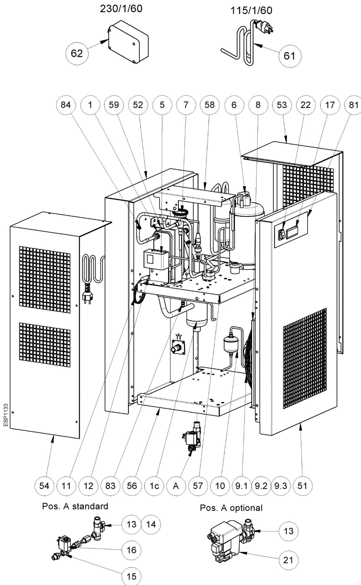
13.2.5 Exploded diagram DRYPOINT RS 180-350 HP50 NA Air-Cooled
