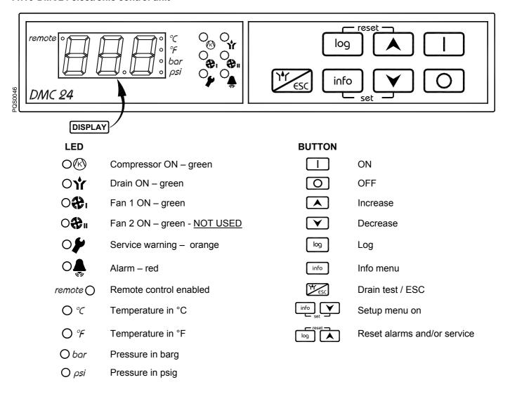
The DMC24 controls all operations, alarms and instrument settings of the dryer. The display and the LEDs indicate all operating conditions.
