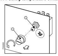
To ensure the operational safety and the soundness of the dryer, a safety temperature switch (TS) is installed at the refrigeration cycle. In the event that the pressure gas temperature is too high, the sensor of the temperature switch will stop the refrigerating compressor to prevent the pressure gas temperature getting too high.
