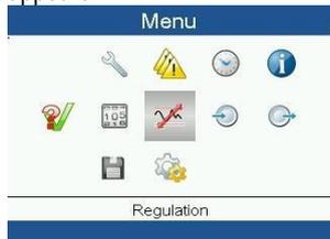
The screen shows a number of icons. Each icon indicates a menu item. By default, the Pressure Settings (Regulation) icon is selected. The status bar shows the name of the menu that corresponds with the selected icon. Use the Scroll keys to select an icon. Press the Escape key to return to the Main screen.
