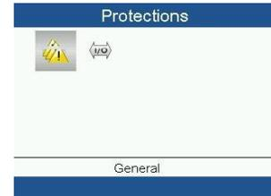
To check which is the shutdown, highlight the red icon, using the Scroll keys. Press the Enter key and it will appear the Protections menu as in picture above in the right side. Press Enter key and then in the display will appear the list of the Protection that are active on the controller. Use Scroll key to check all the protections and the one who is causing the shutdown will be highlighted as in picture below:
