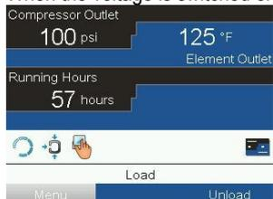
To go to the Menu screen, highlight the Menu button (4), using the Scroll keys. Press the Enter key to select the menu. Following screen appears:
