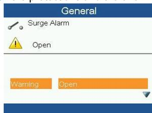
The warning "Surge Alarm" appears when a cartridge of the surge protector device (F99) blown; replace it as soon as possible in order to avoid damages to the frequency converter. (valid only for cULus cubicles). "Only for compressors VSD"
