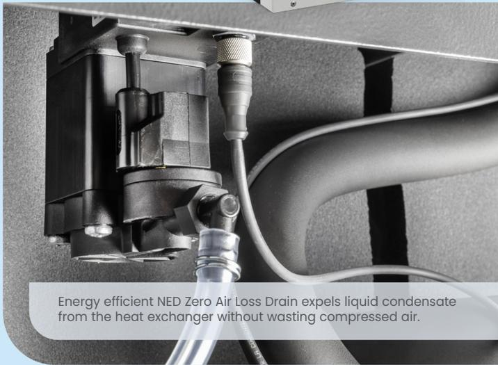
Energy efficient NED Zero Air Loss Drain expels liquid condensate from the heat exchanger without wasting compressed air.
