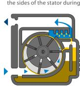
offers remarkable advantages, first among them being **greater volume yield** because the vanes are in constant contact with the inner wall o the stator and form a perfectly airtight seal with no leaks along the wall thanks to a continuous film of oil. In this type of compressor no axial thrust
