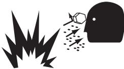
HIGH PRESSURE AIR. Rusted tanks can cause explosion and severe injury or death. Receiver under pressure. Operator should relieve tank pressure before performing maintenance. In addition to automatic drain, operate manual drain valve weekly. Manual drain valve located at bottom of the tank.
