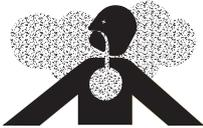
INTAKE AIR. Can contain carbon monoxide or other contaminants. Will cause serious injury or death. **Ingersoll Rand** air compressors are not designed, intended or approved for breathing air. Compressed air should not be used for breathing air applications unless treated in accordance with all applicable codes and regulations.
