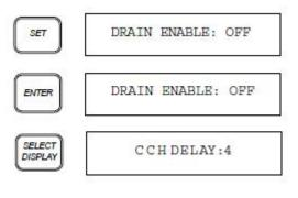
For parameters with "ON / "OFF" or "Y" / "N" choices, the set point is changed using the SET button. Pressing the SET button changes the Drain Enable from ON to OFF.
