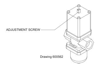
Figure 3 - Water Regulating Valve
