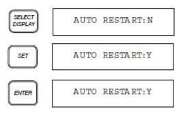
For parameters with "ON / "OFF" or "Y" / "N" choices, the set point is changed using the SET button. Pressing the SET button changes the Drain Enable from ON to OFF.
