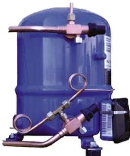
Heavy duty, industrial service piston type refrigeration compressor with proven durability that is designed to handle the fluctuating loads of a compressed air refrigeration dryer. The compressor is equipped with an oil sight glass to verify lubrication levels as well as proper gas return operating conditions. Rotolock service valves allow isolation as well as access to the refrigeration system that aids in the long term service and maintenance of a refrigeration dryer.
