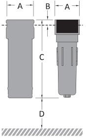
(1) ¼" to 1" NPT maximum design operating pressure 725 psig at 248°F with full CRN certification. Other connections 580 psig at 248°F with full CRN certification, 640 psig at 248°F with no CRN certification. For all other pressures, refer to the pressure correction factor table above
