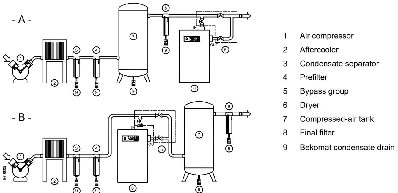
Installation **type A** is recommended when the total consumption corresponds to the throughput rate of the compressor. Installation **type B** is recommended when the air consumption constantly varies, with peak values which considerably exceed the throughput rate of the compressor. The storage capacity of the tank must be dimensioned in such a way that a possible short-term high air demand (peak air consumption) can be compensated.
