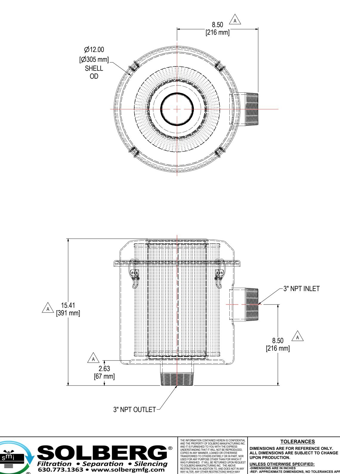
UNLESS OTHERWISE SPECIFIED: -DIMENSIONS ARE IN INCHES -REF: APPROXIMATE DIMENSIONS, NO TOLERANCES APPI -FINISH: BREAK EDGES TO .005-.020 RADIUS/CHAMFER
