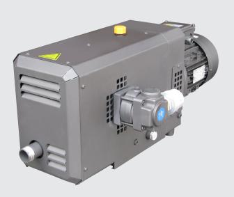
The Airtech VCX positive displacement rotary claw design is air cooled, dry-running and noncontacting. These features, along with quality construction results in a vacuum pump that is extremely high in reliability and a long service life. The non-contact design eliminates internal wear and maintenance. No water levels to check due to air-cooled operation and no sealing or lubricating oil is needed in the pumping chamber.
