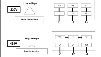
The motor must be connected in accordance with electrical codes through a fused switch in order to protect the motor against electrical or mechanical overload conditions. The overload of the motor starter must be set at a level equal to the full load motor current listed on the motor nameplate.
