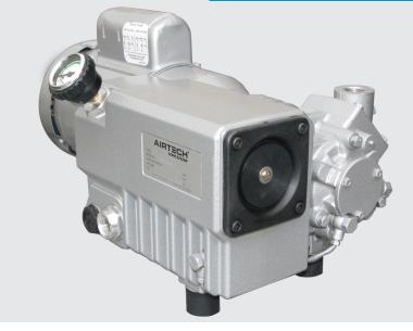
Airtech's L-Series rotary vane oil-flooded vacuum pump is a real workhorse. Reliability and durability are ensured by its simple design. Our L-Series Pump has integral exhaust filters, vibration isolators, and composite vane material which promotes longevity. The Airtech pump has an operating capacity range of 7-460 CFM while obtaining an end vacuum of 0.5 Torr.
