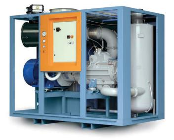
**Airtech's ATV** rotary vane vacuum pumps are rugged, single stage, air-cooled, and direct drive. Its high efficiency design provides performance equal to larger vacuum pumps but with lower energy usage. These vacuum pumps offer ease of installation, automatic operation, and achieve deep vacuum level to 2.0 mm HgA. Pumping speed remains consistent through a wide vacuum range. The deep vacuum capability makes it suitable for a wide range of applications across many industries.
