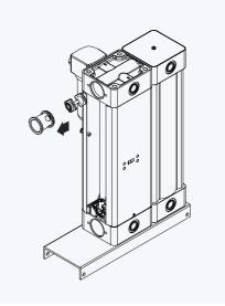
Figure 6.31: 45 SCFM - 365 SCFM Shuttle seat and shuttle removal (Bottom block)
