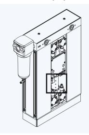
Figure 6.16: 4 SCFM - 35 SCFM Silencer changout stage 2
