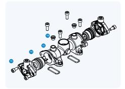
Fig 11.11 Bottom valve block assembly
