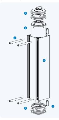
Fig 11.5 Top tower plug assembly
