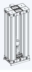
Figure 6.22: 215 SCFM - 365 SCFM Silencer changout stage 2
