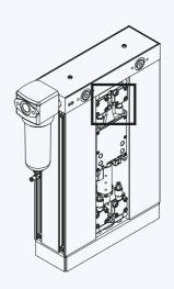
Figure 6.12: 4 SCFM - 35 SCFM - Purge plug changeout stage 2
