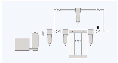
To prevent back flow into the dryer a non-return valve should be placed in-line, downstream of the dryer. This is essential when more than one dryer is used in a single application.
