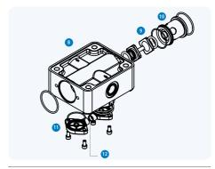
Fig 11.10 Exhaust manifold assembly
