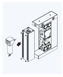
Figure 6.28: 4 SCFM - 35 SCFM Shuttle seat and shuttle removal
