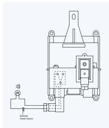
Remote alarm wiring diagram
