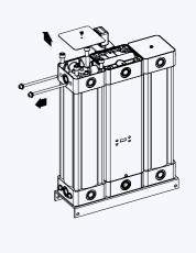
Figure 6.8: Models 45 SCFM - 365 SCFM - QPM removal stage 2
