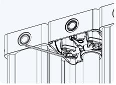
Figure 6.14: 45 SCFM - 365 SCFM Purge plug change out stage 2
