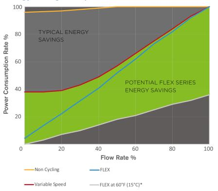
Dryers are rated in a accordance to ISO 7183 standard rating conditions A2. (38°C / 100°F ambient)
